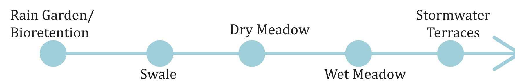
Our Treatment Train filters water through a variety of LID controls
