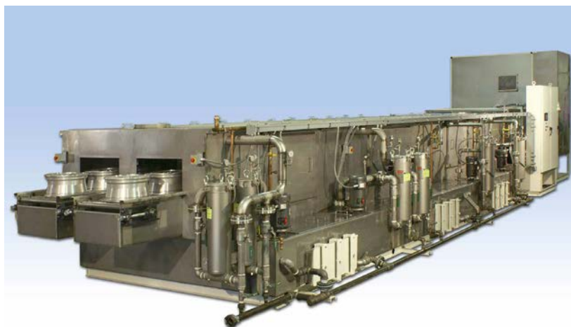
Figure 2-8. Belt/Strip Conveyorized Degreaser (USEPA 1977)
