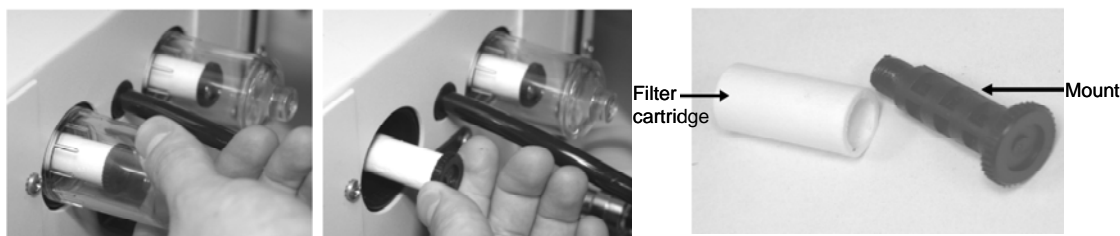
Figure 10-3. The PM 2.5 and PM-Coarse in-line filters should be changed every six months.
