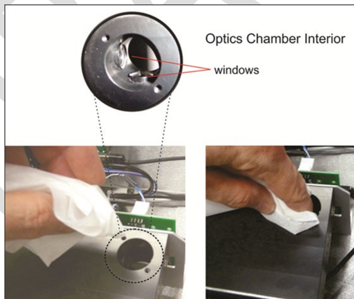
Figure 8. Maintenance: Optics Chamber Windows.
