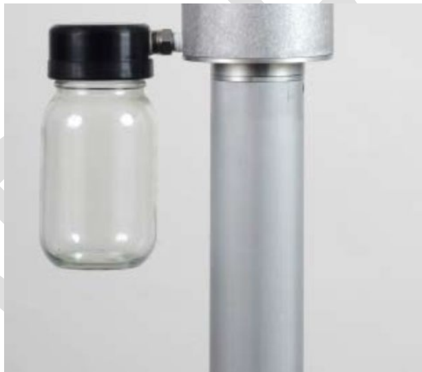
Figure 20. Water Collector Attached to Inlet.
