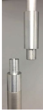
Figure 11. Slip coupler moved to the side to allow monitor use with audit devices.
