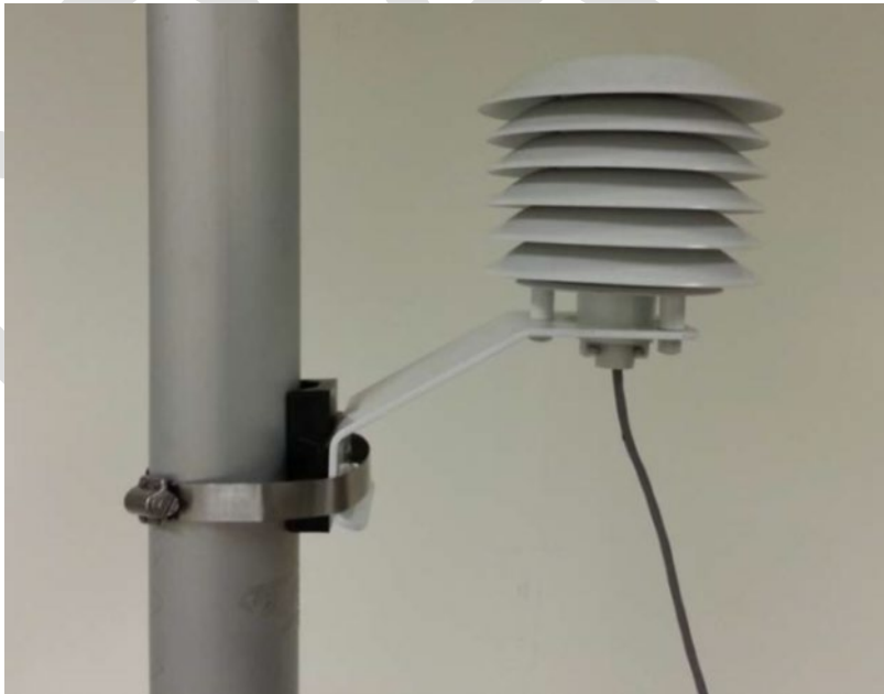
Figure 23. Ambient Temperature Probe Installed in Solar Shield.
