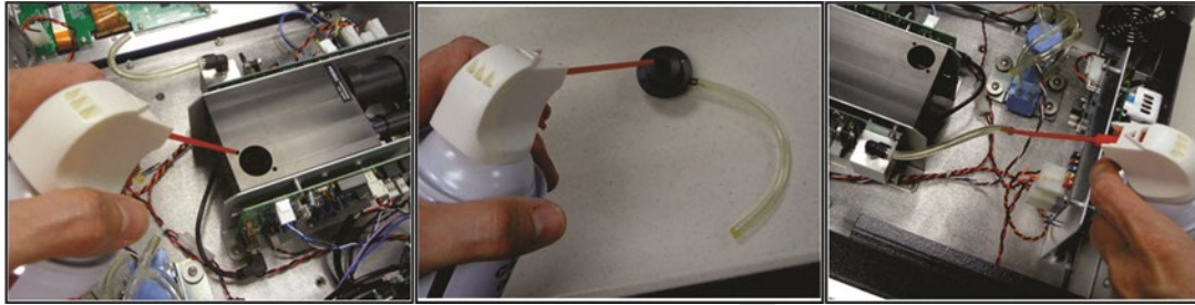
Figure 9. Maintenance: Final Dusting.
