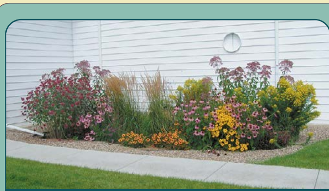
A rain garden at the North Great Plains Research Laboratory near Bismark ND uses native plants to absorb and filter stormwater and return it to the groundwater system.
