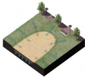
■ □ □ Surface Sand Filters
