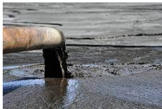
Photo 2: Slurried Coal Ash Being Discharged to a Management Unit Credit: U.S. EPA
