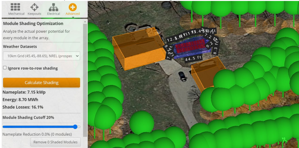
Figure 19: Shade loss analysis for a moderate shade home. Analysis performed in Helioscope.
