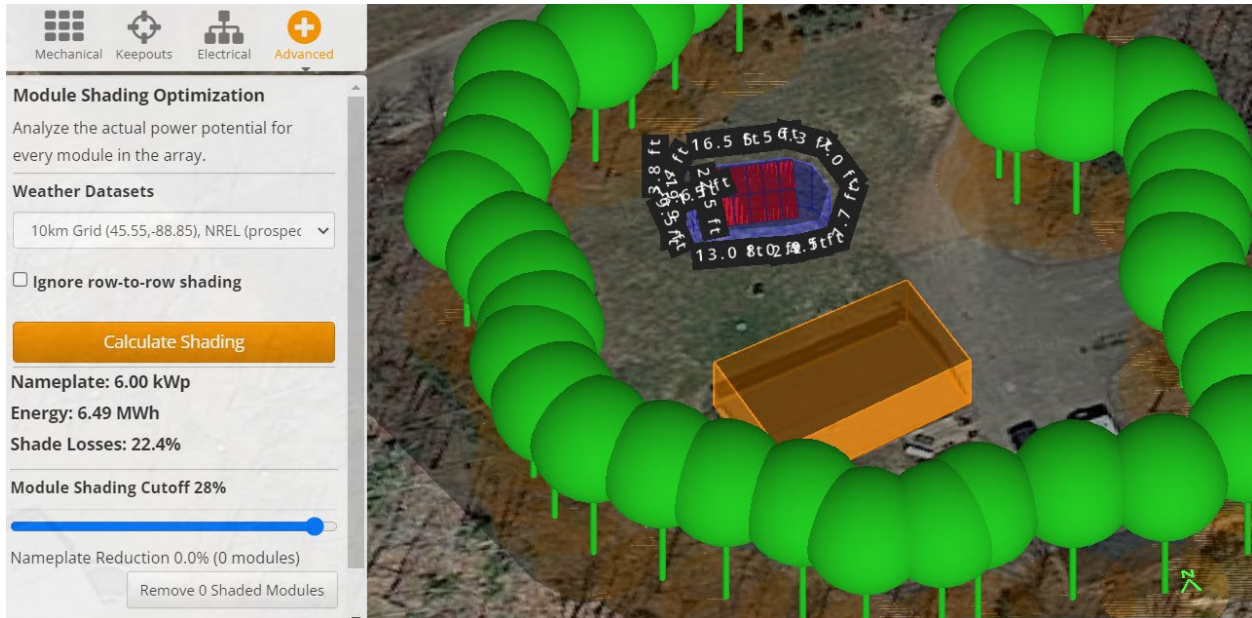
Figure 20: Shade loss analysis for a high shade home. Analysis performed in Helioscope.
