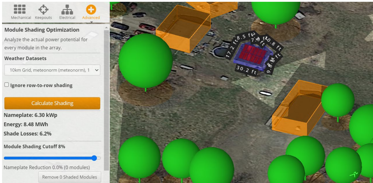
Figure 18: Shade loss analysis for a low shade home. Analysis performed in Helioscope.
