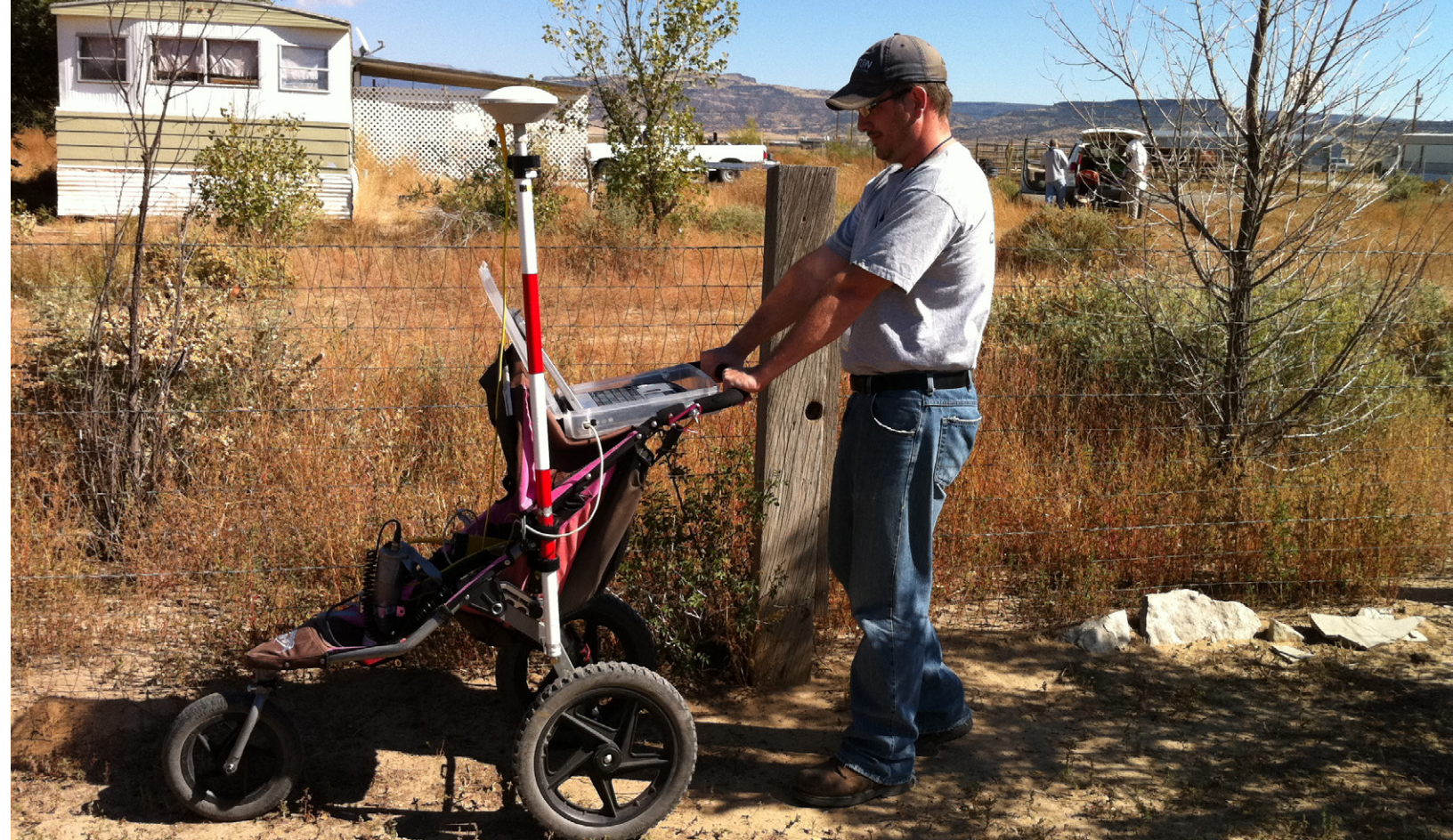
EPA Contractor conducting a residential gamma survey. The buggy contains GPS and measuring instruments.
