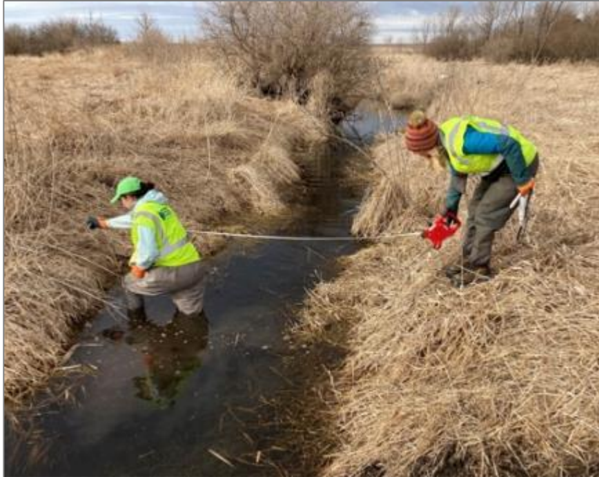
Figure 5. Measuring bankfull width. Image credit: James Treacy
