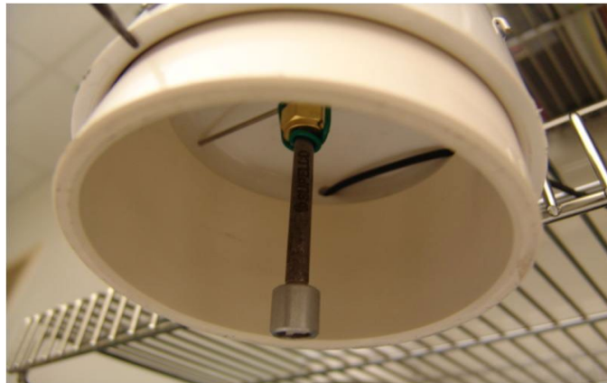
PS Sampler Example PVC Pipe version with weatherproof hood
